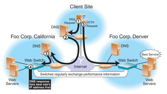
Figure 12-1 DNS Resolution with Global Server Load Balancing
